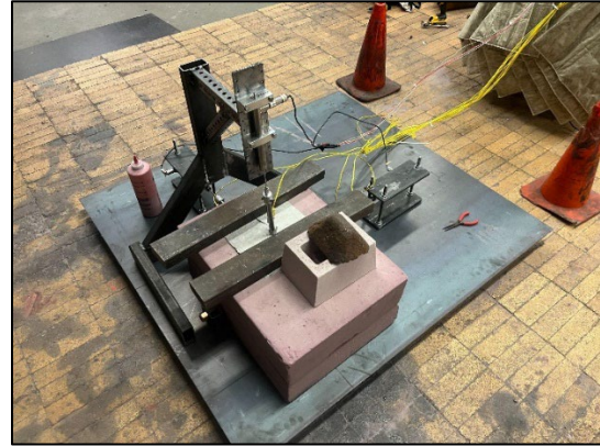
Figure 8. Instrumented mold prepared with all sensors connected, prior to the installation of sensor shielding.
