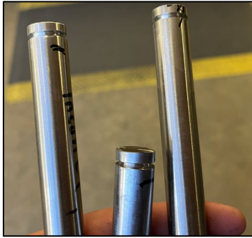
Figure 3. Inconel push rods with machined grooves to ensure connection between casting and pushrods.
