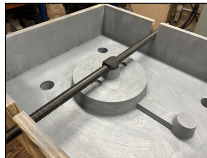
Figure 6. Drag pattern with fixture rod inserted prior to molding.
